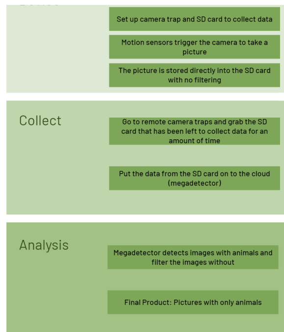
Figure 2: Current method used by Zelmer, 2020 including megadetector.
