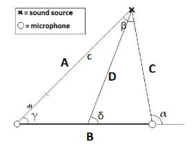
between sound signals to find a source angle. The code uses a threshold value to detect sounds over that value and interpret them as peaks. These signals are recorded and then the software find the time difference between two peaks. The speed of sound is theoretical so as to obtain values by tapping the microphone. The slope of a singular line is outputted.
