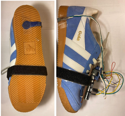
Figure 5. Final prototype- Force Sensor with Accelerometer and Arduino.
